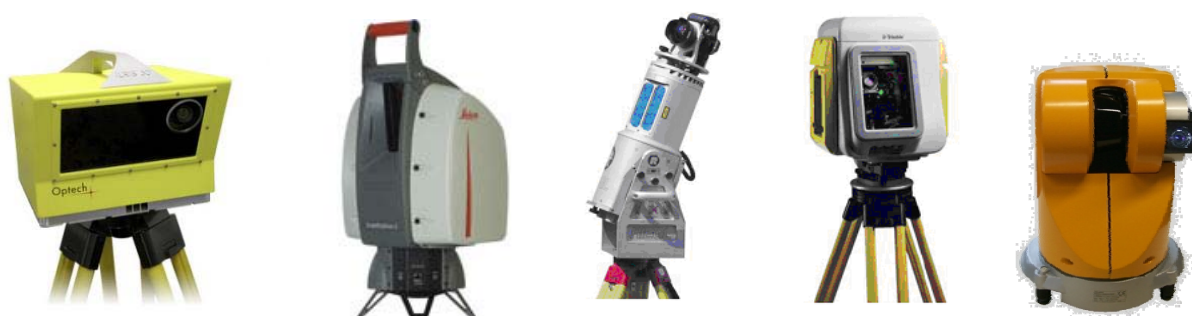
Figuur 15: Commercieel beschikbare Time-Of-Flight Laser Scanners
