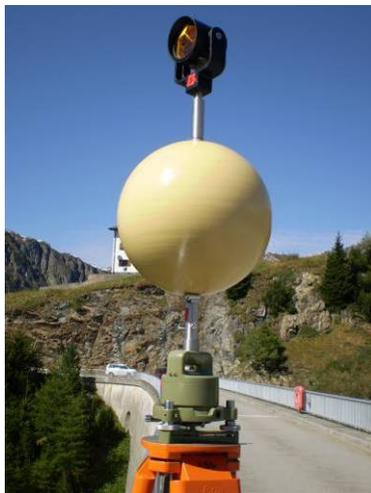
Figure 212: Painted wooden sphere with prism assembly,  $d=23.85\text{cm}$
