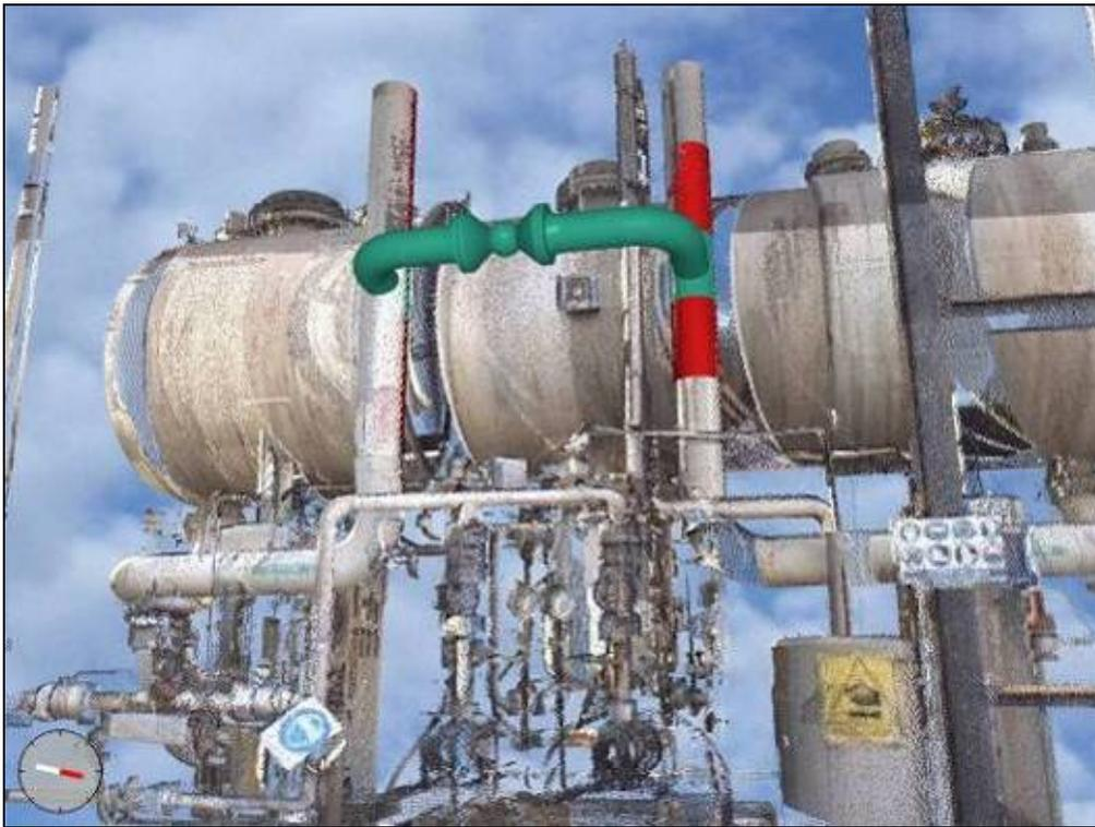
Figure 183: Hybrid 3D review using Navisworks - © BnS engineering N.V.
