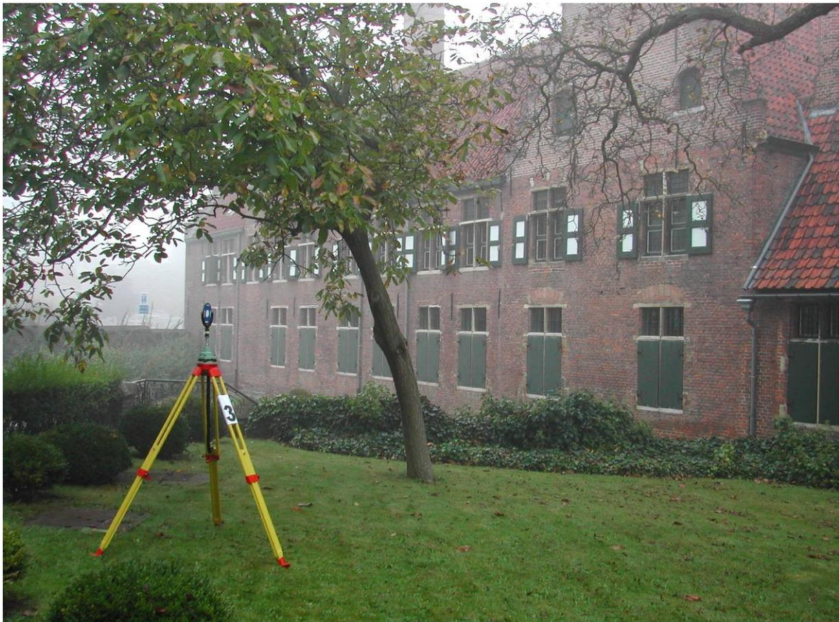
Figure 39: Scanning artificial targets
