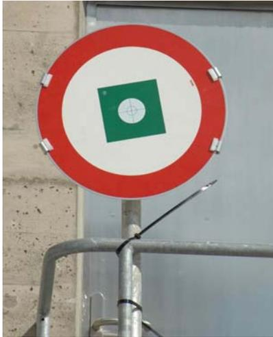
Figure 210: Flat target in Traffic sign
