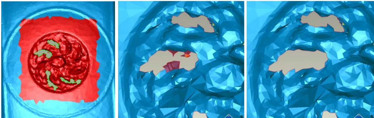
Figure 126: Cleaning hole boundaries before filling
