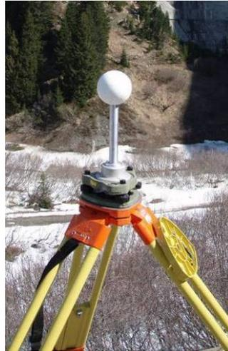
Figure 211: Trimble sphere,  $d=7.6\text{cm}$  and interchangeable prism
