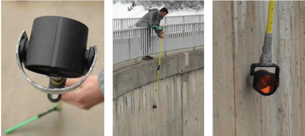
Figure 215: Tachymetric measurement of the dam crest
