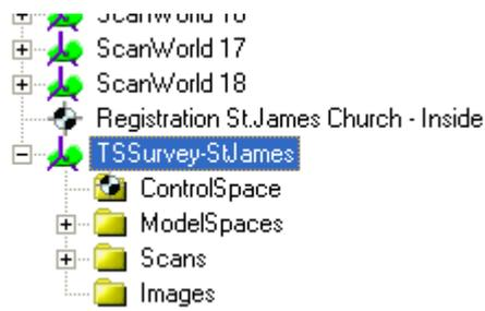
Figure 65: Structure of the imported total station data in Cyclone
