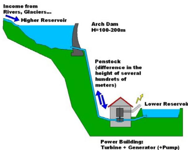
Figure 190: Pumped storage plant (Schematic)
