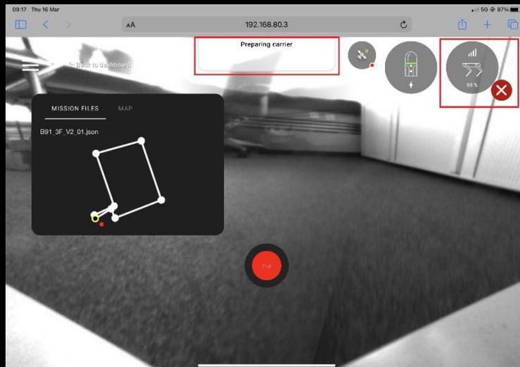
After powering on the carrier, the robot control panel appears. Use the remote joysticks to move the robot within the range where the fiducial can be detected.
