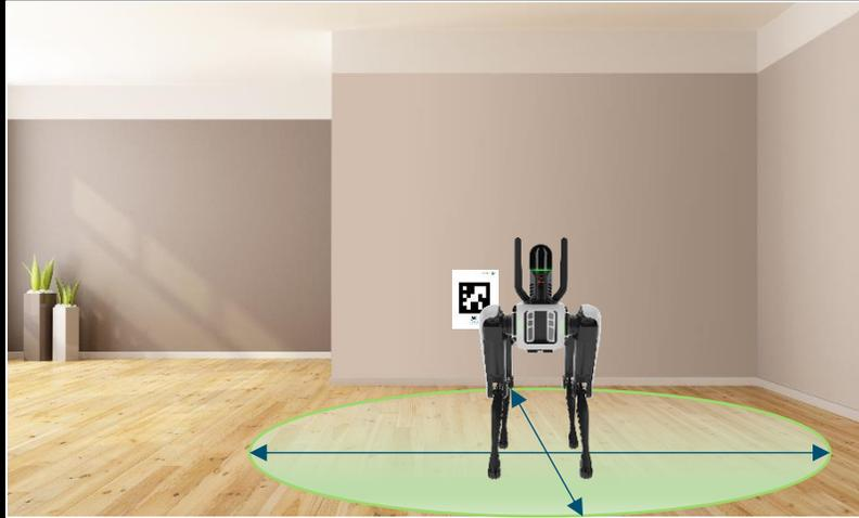
Thanks to that BLK ARC will be positioned a bit further away from walls and possible obstacles, which will allow for capturing good quality data for better SLAM initialization. Please note that for BLK ARC LiDAR the minimum measuring distance is 50 cm.
