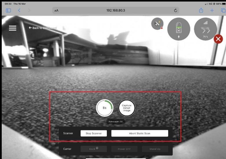
Make sure there is enough space around the robot during the static scans as the robot will move to the tripod position. During a static pose, the manual control panel will disappear to prevent unintentional movement commands. The countdown till the end of the static scan will be displayed. During tripod pose, the robot's collision avoidance is working and in rare cases, when collision is
