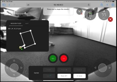
During the mission, the operator can **Pause** or **End** the mission. While the mission is paused, the **control panel** for the robot appears. The operator can manually move the robot and **Resume** the mission anytime. Please note, that in this case the BLK ARC module is continuously collecting the data.
