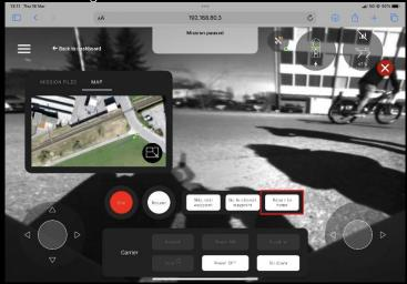
The **Return to Home** command will be executed automatically when the carrier will reach an obstacle on its path and will not be able to avoid it.
