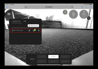
Press marked icon in order to upload & attach a 3D map to your mission file. **Note**: Icon for attaching 3D map is disabled if 3D model is not attached yet.
