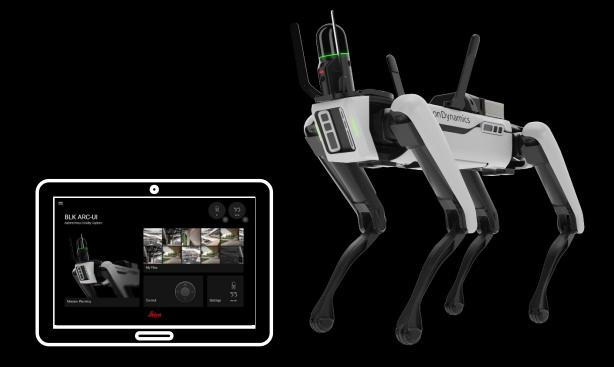
BLK ARC-UI is a browser-based user interface dedicated for operating BLK ARC Laser Scanner integrated by Leica Geosystems with robotic carriers, such as Boston Dynamics Spot robot.
